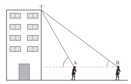
From position B, the angle of elevation to T at the top of the tower is  $64^{\circ}$ . From position A, the angle of elevation to T at the top of the tower is  $69^{\circ}$ . The distance AB is 4.8 metres and the height of the student to eye level is 1.5 metres.
