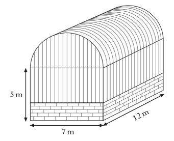
The cross-section of the storage barn consists of a rectangle measuring 7 metres by 5 metres and a semi-circle of radius 3.5 metres.
